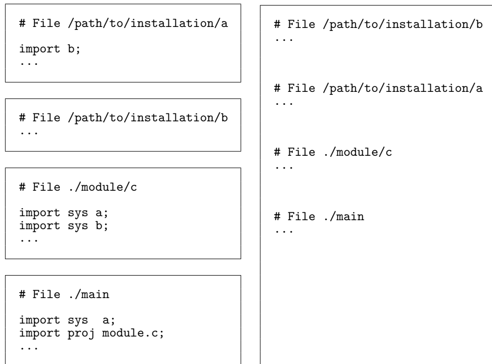
Figure 4.10: Compilation of file ./main . Imported files are prepended in topologically sorted order.
